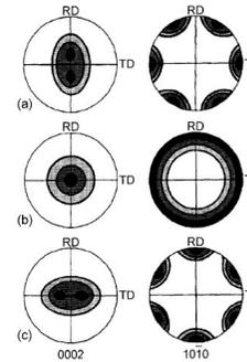
Fig. 22. Schematic rolling textures in hcp metals with  $c/a$  ratios of (a) greater than 1.633, (b) approximately equal to 1.633 and (c) less than 1.633. 0002 and 1010 pole figures. (TINCKHOFF 1988).
