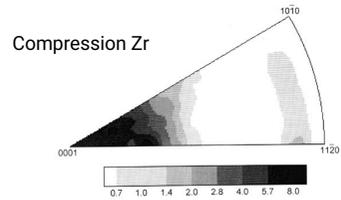
Fig. 21. Inverse pole figure (plate normals) for forged and cross-rolled zirconium.
