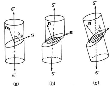
Fig. 10.5 Rotation of crystal lattice in tension
