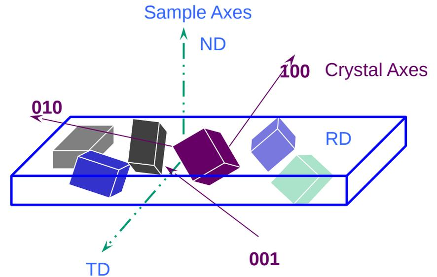
Rotation 1 ( $\phi_1$ ): rotate sample axes about ND
