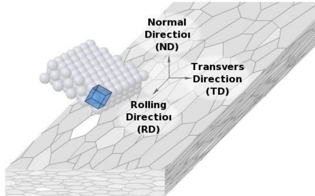
Cubic-structured crystallite in a deformed sample
